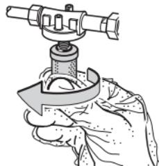
Hold the new filter cartridge by the upper plastic part and screw it in **by hand** (max. 1.5 Nm)
